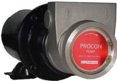
Due to the elimination of the mechanical seals, PROCON's family of MagDrives provides you with a virtually leak proof pump. They are designed for those applications which use a "hard to contain" fluid (e.g. glycols, oils, low surface tension fluids, etc.). PROCON's Series 6 MagDrive is designed and built to meet your needs for higher flows. The flow rate capacity for this pump ranges from 300 to 660 gallons per hour at 250 psi. No integral relief valve is available.
