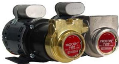
Due to the elimination of the mechanical seals, PROCON's family of MagDrives provides you with a virtually leak proof pump. They are designed for those applications which use a "hard to contain" fluid (e.g. glycols, oils, low surface tension fluids, etc.). PROCON's Series 2 and 3 MagDrives are available in 11 flow rates: 15, 25, 35, 50, 60, 70, 80, 100, 110, 125 and 140 gallons per hour with discharge pressures up to 180 psi. Brass or stainless steel construction is available.
