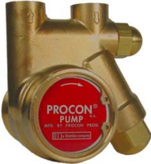
PROCON's Series 1 pumps have the protection of an integral inlet strainer. The standard strainer is a 100 mesh wire screen. It traps particles that can cause serious damage to the pump. The strainer is equipped with a removable cap to allow periodic cleaning, every 4 months under normal conditions (more frequently with hard or turbid water). The clamp-on mounting style is shown in the photo; bolt-on mounting is also available.
